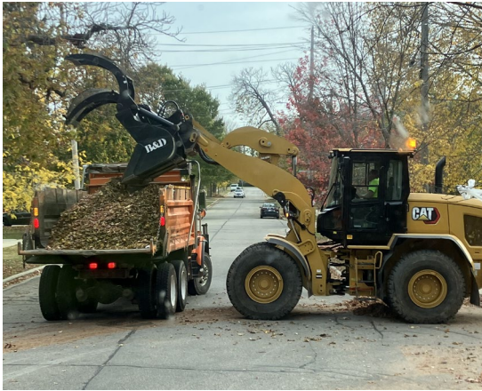
(Loader with grapple loading leaves)
